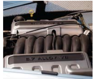
■ ABOVE The spare wheel leaves little spare room in the boot. ■ BELOW The Spyder's LS1 Chevrolet V8 hooks up to a four-speed automatic transmission.
